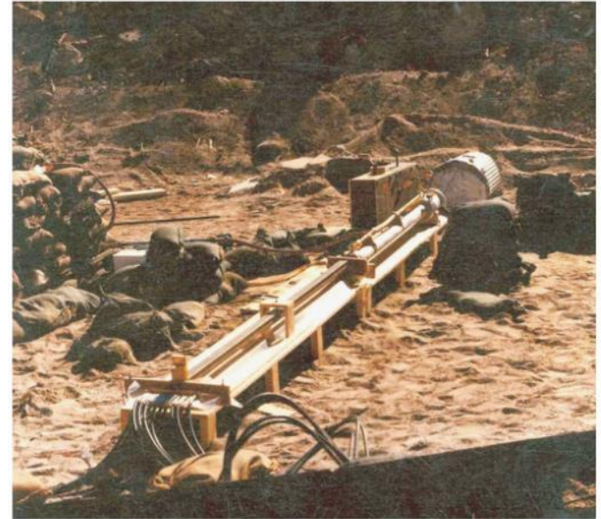
Fig. 30. Strip generator powered railgun at Ancho Canyon firing site (LANL).
